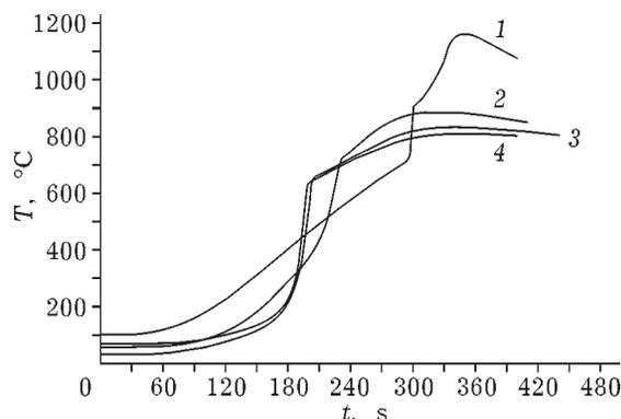
Fig. 1. Thermograms of thermal explosion of the initial (1) and mechanically activated samples 3Fe + Al (2–4). Time of mechanical activation, s: 10 (2), 60 (3), 140 (4).
