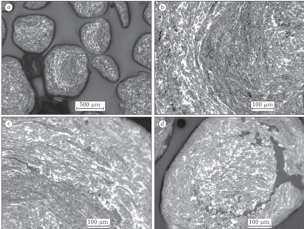
Fig. 3. Microstructure of mechanocomposites activated for 150 s: *a* - general view, *b* - layered structure, *c* - long cracks, *d* - intensive formation of cracks as a result of the application of MA.
