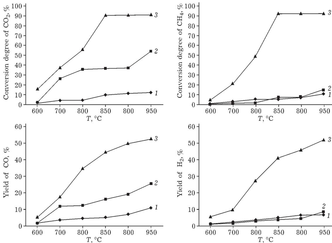
Fig. 5. Catalytic data obtained in the process of carbon-dioxide conversion of methane ( $v(\text{CO}_2 + \text{CH}_4) = 100 \text{ mL/min}$ , catalyst volume  $1 \text{ cm}^3$ ) for the samples having the composition Fe (1) and Fe + 13.7 mass % Al after SHS (2) and after MA for 2.5 min and SHS (3).
