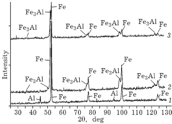
Fig. 2. X-ray diffraction patterns of reaction mixtures: 1 - Fe + 13.87 mass % Al after MA for 2.5 min before SHS; 2 - 3Fe + Al after SHS without MA; 3 - 3Fe + Al mechanically activated of 2.5 min after SHS.
