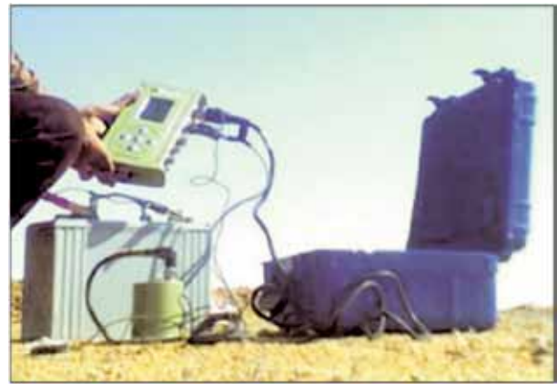
Fig. 4. Taurus seismograph with Trillium 120s seismometer for microtremors recording are in use.
