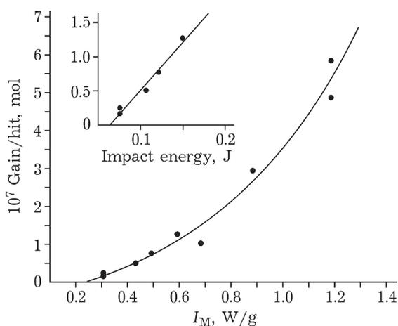
Fig. 5. Increase in the mechanochemical gain per hit ( $g_m$ ) as a function of the milling intensity ( $I_M$ ). Inset: mechanochemical gain vs. impact energy for experiments carried out at the same impact frequency.
