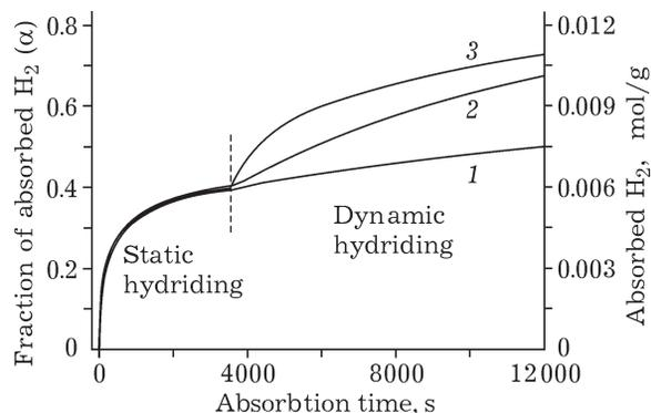
Fig. 4. Hydriding process for the  $\text{Mg}_2\text{Ni}/\text{Ni}$  nanocomposite: absorption under conventional thermal activation (left side) was followed by trials carried out under milling conditions at the quoted  $I_M$  values,  $\text{W}/\text{g}$ : 0.31 (1), 0.61 (2), 0.88 (3).
