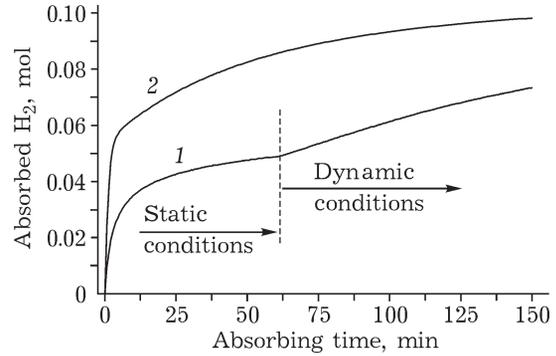
Fig. 3. Absorbed hydrogen moles for  $\text{Mg}_2\text{Ni}/\text{Ni}$  powder samples as a function of the elapsed time: 1 – collected under static absorbing conditions up to the marker, then under milling; 2 – the process carried out under milling from the beginning.  $I_M = 0.68 \text{ W/g}$ .
