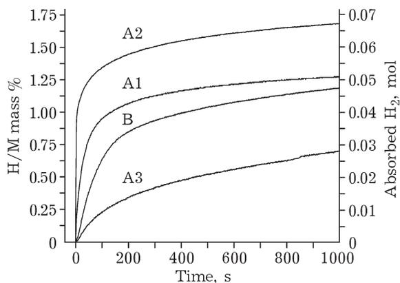
Fig. 1. Hydrogen absorbing kinetics for the nanosized A1, A2, A3 and B samples characterized in Table 1. Irrespective to preparation mode the hydriding process is deceleratory throughout.
