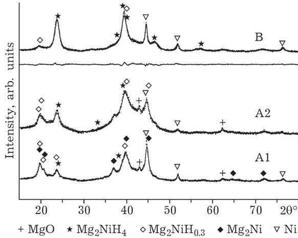
Fig. 2. XRD patterns of the  $\text{Mg}_2\text{Ni}/\text{Ni}$  samples after the first hydriding run. Irrespective to the sample preparation techniques,  $\text{Mg}_2\text{NiH}_{0.3}$  and traces of monoclinic hydrogen-rich  $\text{Mg}_2\text{NiH}_4$  result in the samples subjected to static hydriding runs – lower patterns. In the upper pattern, which refers to a B-type sample charged by reactive milling, the hydrogen-rich  $\text{Mg}_2\text{NiH}_4$  is the prevailing hydride phase.
