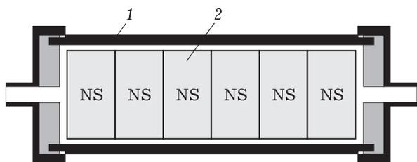
Fig. 1. Scheme of MAUT device: 1 – housing, 2 – magnetic system.
