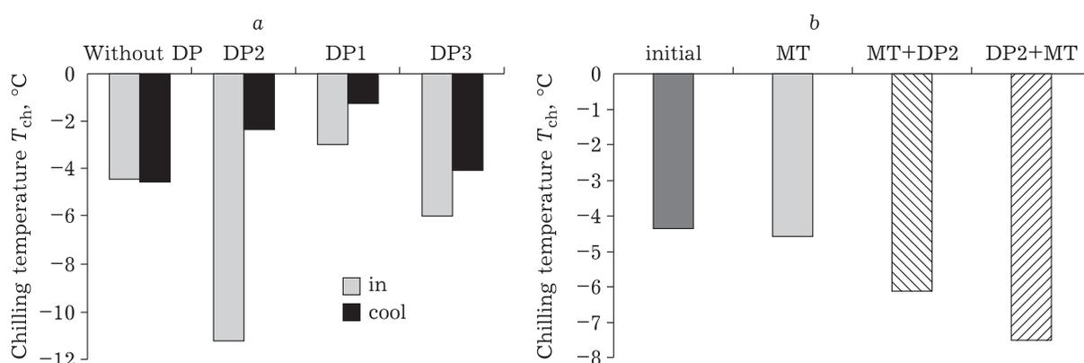
Fig. 3. Comparison between chilling temperatures of non-thermostated (in), thermostated (cool) oil with DP1, DP2 and DP3 additives (a) and oil samples after magnetic treatment (MT) and integrated treatment (b).
