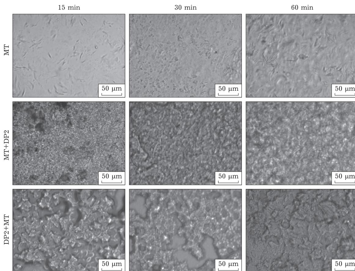
Fig. 5. Microphotograph of sediments isolated from oil in 15, 30 and 60 min after different kinds of treatment.
