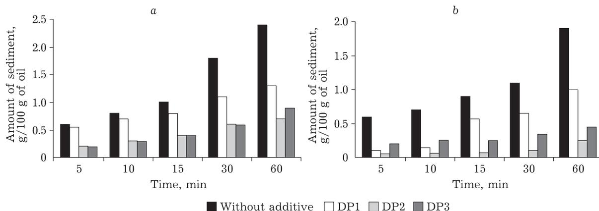
Fig. 2. Effect of DP1, DP2 and DP3 additives on the kinetics of precipitation in initial oil (a) and in oil cooled to 0 °C (b).
