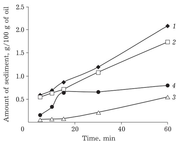
Fig. 4. Kinetics of the formation of precipitate in oil: 1 – initial, 2 – after magnetic treatment (MT), 3 – after integrated treatment MT+DP2, 4 – after integrated treatment DP2+MO.
