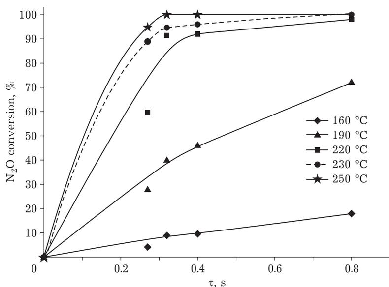
Fig. 3. Dependence of  $N_2O$  conversion on the oxide Ni-Co-containing catalyst on contact time at different temperatures. The graphs were plotted in OriginPro 9.1 software, the curves were approximated by the Akima-Spline function.
