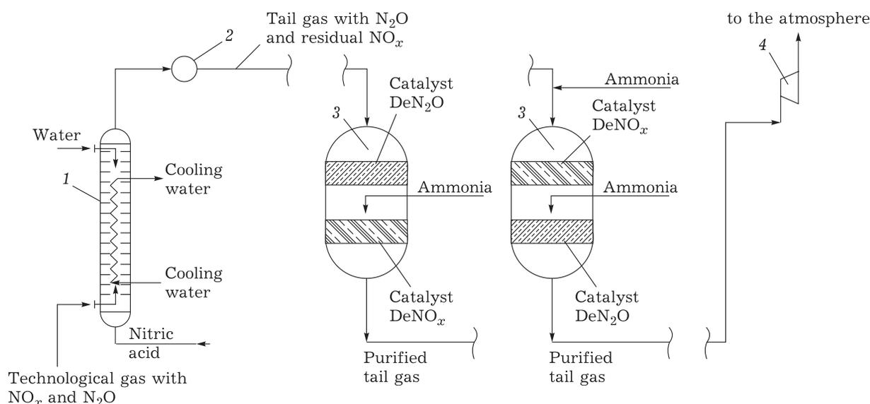
Fig. 1. Scheme of EnviNOx® technology: *a* – version 1 (catalytic decomposition of  $N_2O$  and reduction of  $NO_x$  by ammonia); *b* – version 2 ( $NO_x$  reduction with ammonia and  $N_2O$  reduction by hydrocarbons). 1 – absorption column; 2 – heater of tail gas; 3 – reactor; 4 – turbine of tail gas.
