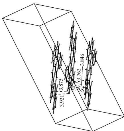
Fig. 3.  $\pi$ — $\pi$  and CH— $\pi$  interactions between infinite parallel layers
