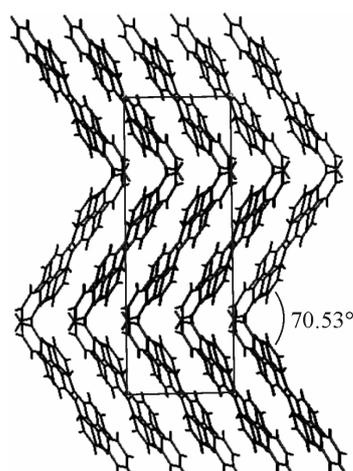
Fig. 4. Two different parallel layers with an angle of  $70.53^\circ$  between the least-squares planes defined by the two entire molecules
