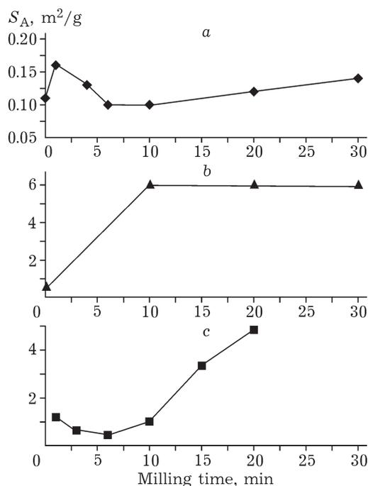
Fig. 8. Specific surface area ( $S_A$ ) vs. milling time: a – copper sulphides; b – silicon; c – mixture of copper sulphides with silicon.
