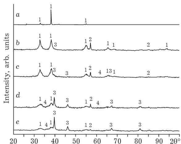
Fig. 4. XRD patterns at different stages of reaction (1) as a function of milling time: a - PbS; b-e - PbS + Fe milled for, min: 20 (b), 30 (c), 40 (d), 60 (e); 1 - lead sulphide, 2 - iron, 3 - lead, 4 - FeS (cubic).
