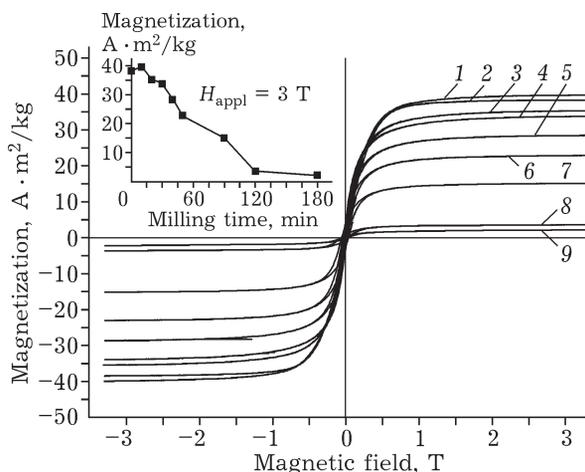
Fig. 5. Magnetization as a function of external magnetic field and/or of milling time for reaction (2). Milling time, min: 0 (1), 10 (2), 20 (3), 30 (4), 40 (5), 50 (6), 90 (7), 120 (8), 180 (9).
