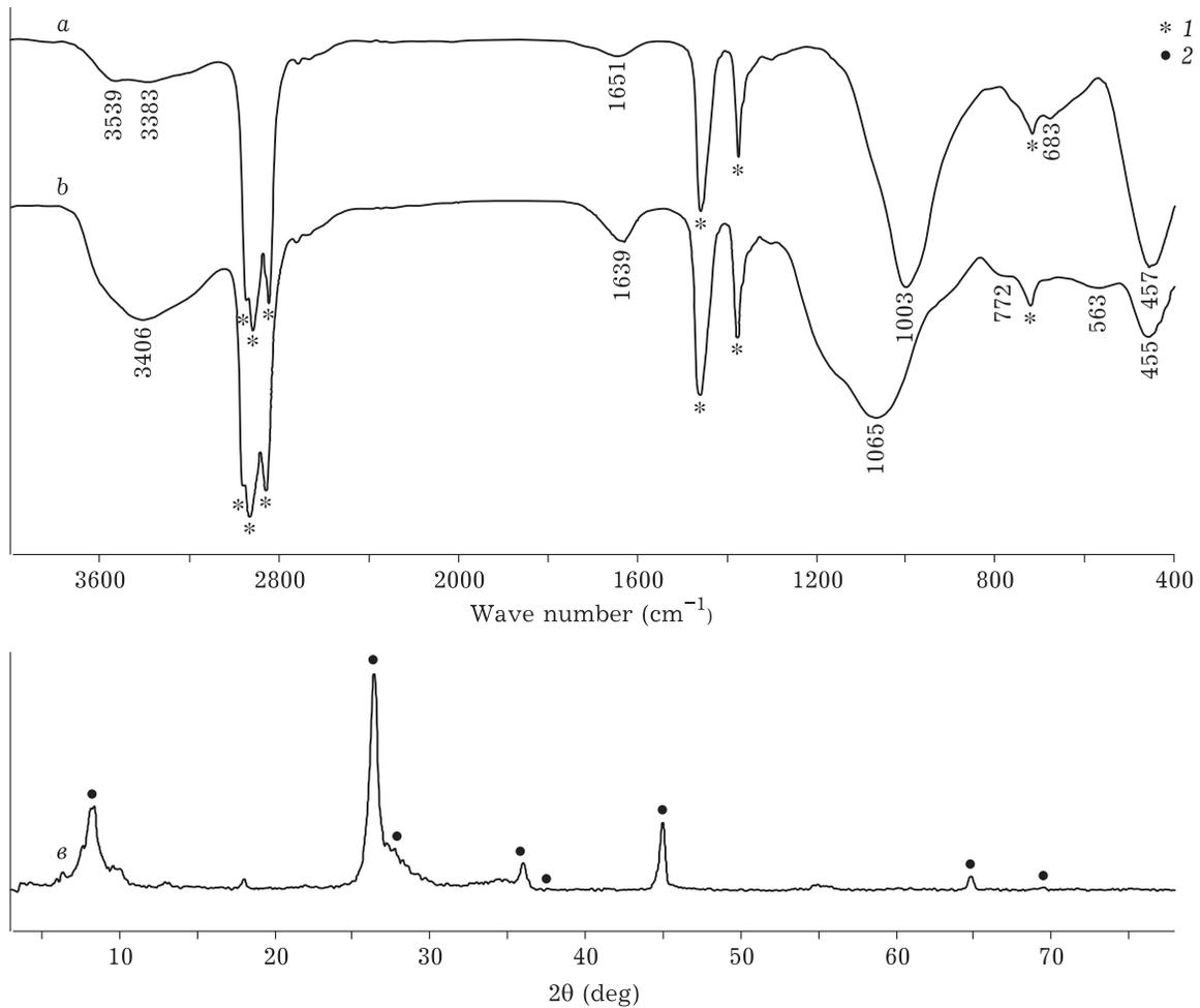
Fig. 2. IR spectrum (a) and X-ray diffraction pattern (c) of vermiculite mineral from the Koksharovskiy deposit and IR spectrum of synthetic aluminosilicate (b) [10]. 1 – absorption bands of vaseline oil; 2 – position of the reflection of vermiculite according to the PDF 2 database.
