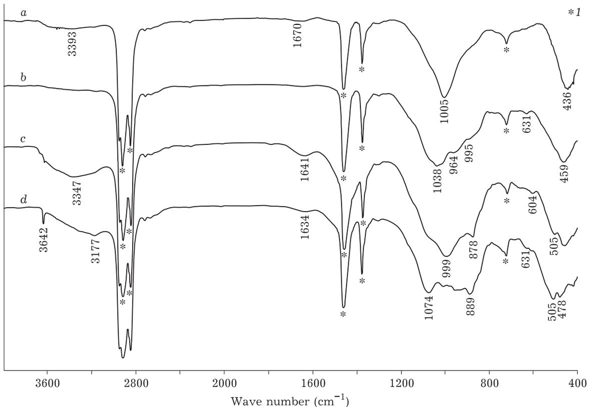
Fig. 4. IR spectra of samples (the <0.05 mm fraction) of expanded vermiculite from Koksharovskiy (*a*, *b*) and Kovdor (*c*, *d*) deposits: *a*, *c* – initial, *b*, *d* – after calcination at 1000 °C. 1 – absorption bands of vaseline oil.
