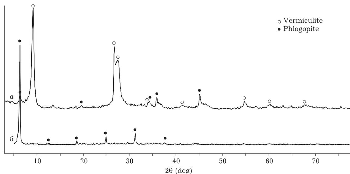
Fig. 3. X-ray diffraction patterns of expanded vermiculite from Koksharovsky (a) and Kovdor (b) deposits.
