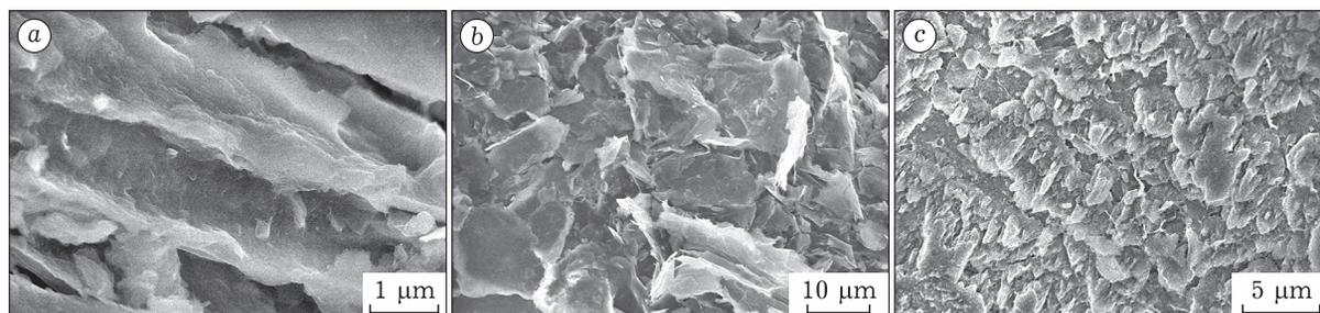
Fig. 1. Micrographs of vermiculite from the Koksharovskiy deposit: mineral (a) and the intumesced product (b) and expanded vermiculite from the Kovdor deposit (c).
