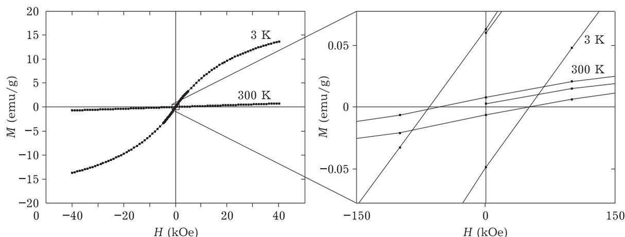
Fig. 5. Field dependencies of magnetization of expanded vermiculite (sample 2) from the Koksharovsky deposit at temperatures of 3 and 300 K.
