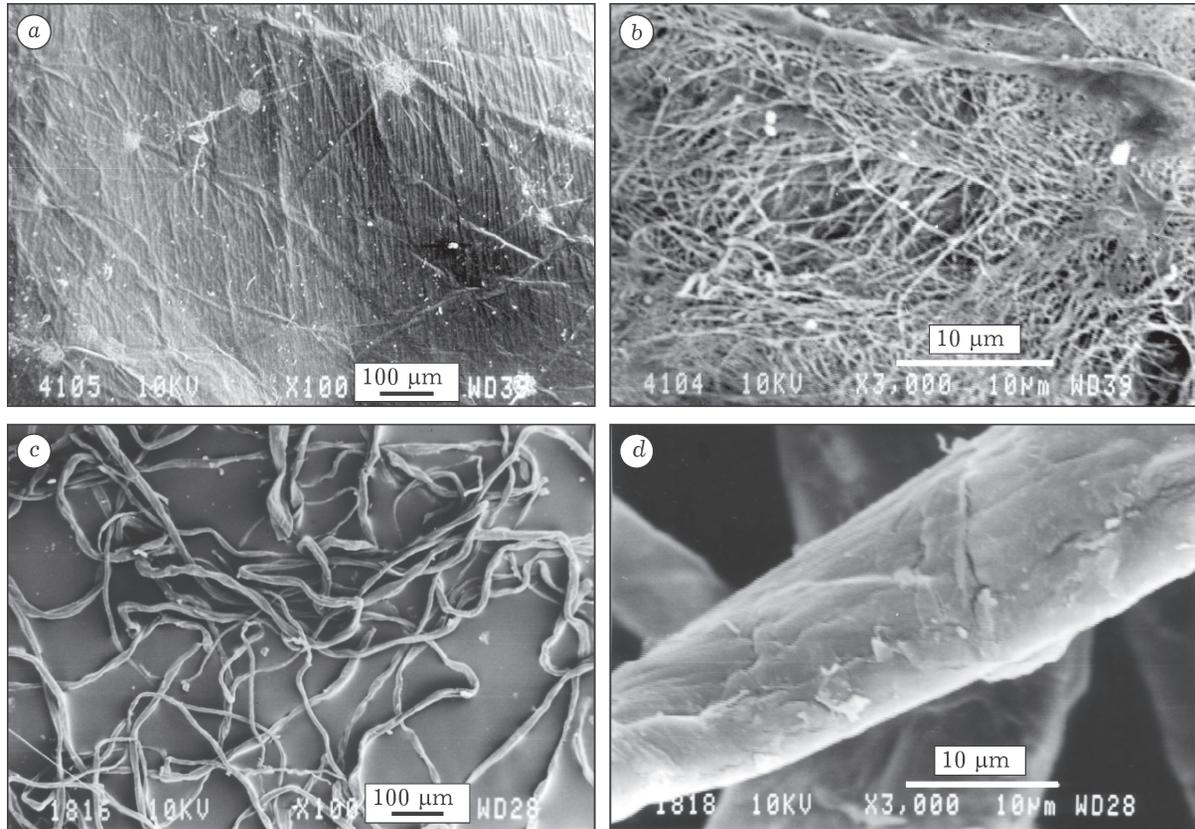
Fig. 2. Photomicrographic images of BCF (a, b) and cotton cellulose (c, d).
