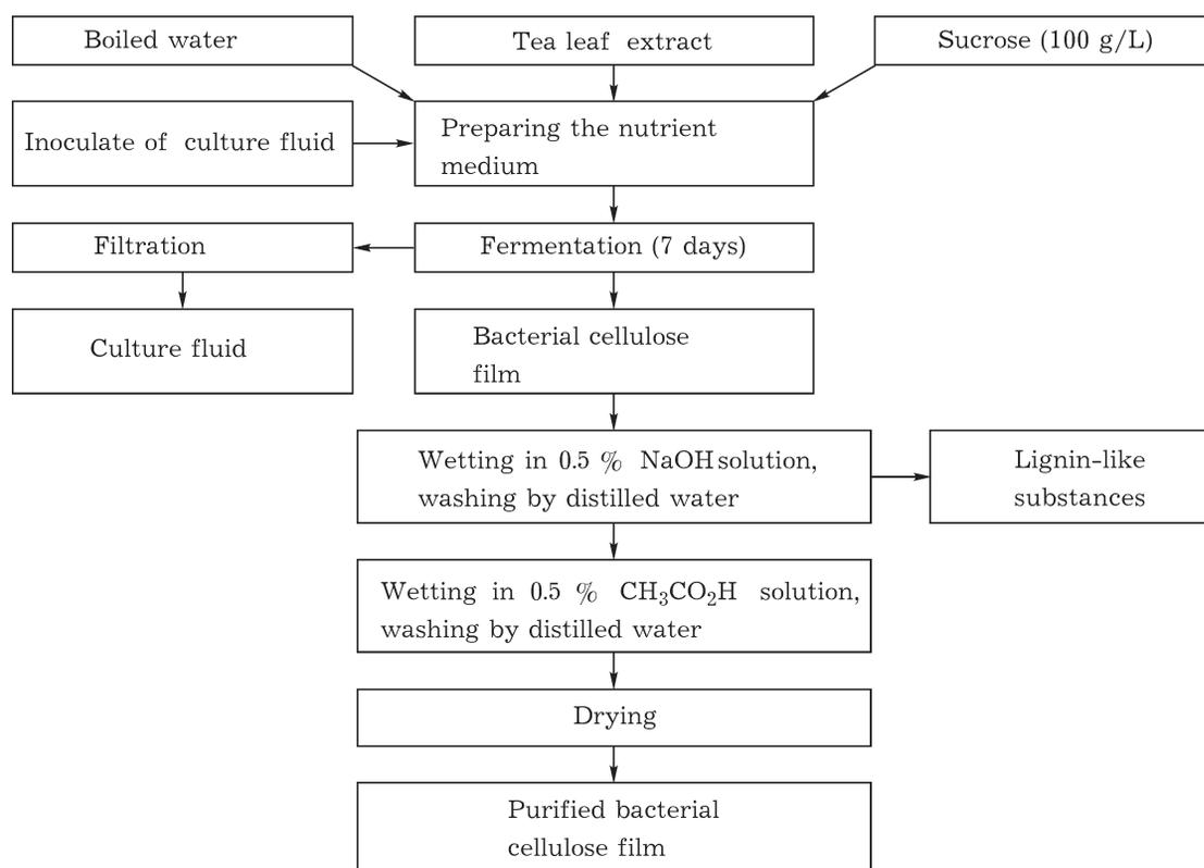
Fig. 1. Block diagram of obtaining the bacterial cellulose film.
