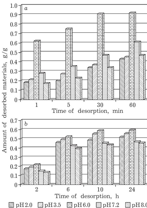
Fig. 4. Kinetics of ACA desorption (a) and sea-buckthorn oil (b) from BCF. The mass of the ACA in the sample before desorption being equal to 1.091 g/g, the mass of sea buckthorn oil in the sample before desorption being equal to 0.597 g/g.
