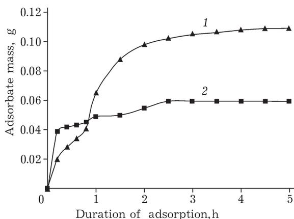
Fig. 3. Kinetics of the adsorption of ACA (1) and sea-buckthorn oil (2) of BCF.
