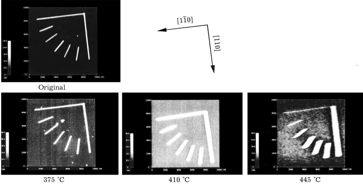
Fig. 6. Table pattern's AFM image before and after MLE.
