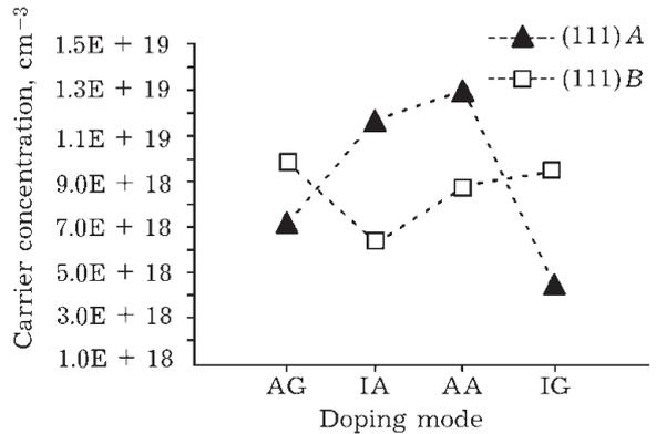
Fig. 4. Carrier concentration of Te doped (111) A (260 °C) and (111)B (383 °C) on each doping modes.  $P$ , Torr:  $10^{-3}(\text{AsH}_3)$ ,  $7.2 \cdot 10^{-6}$  (TEG),  $10^{-7}$ (DET).
