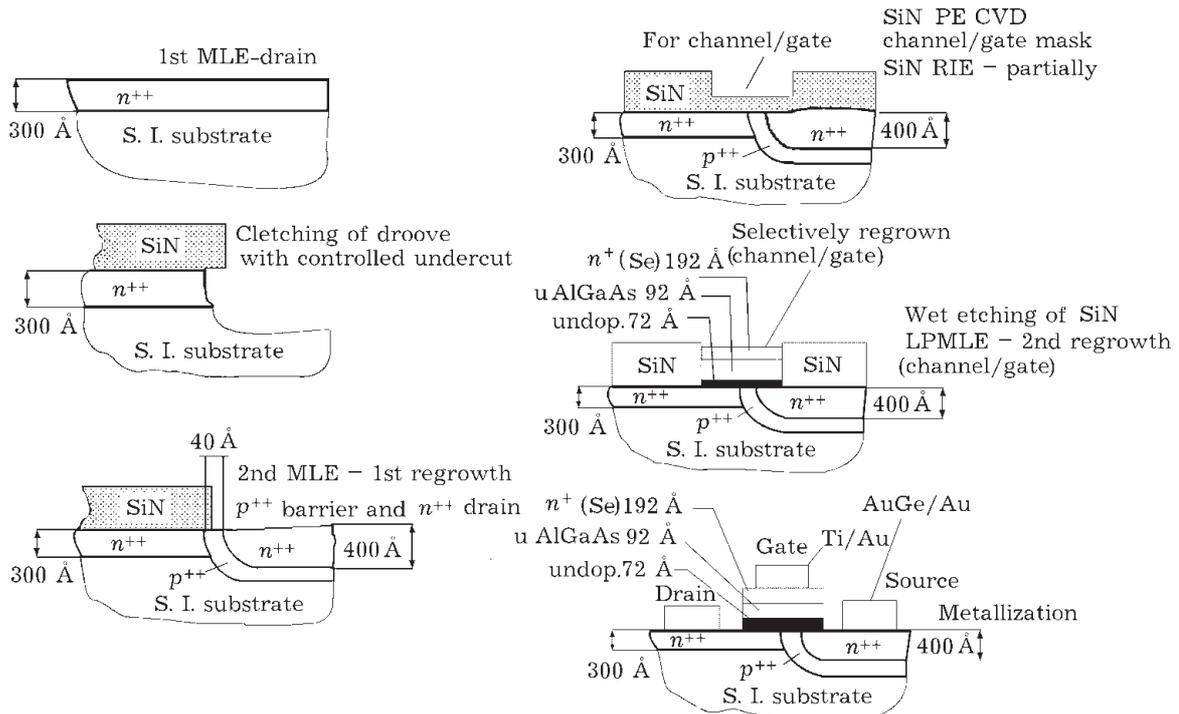
Fig. 1. Fabrication and structure of horizontal ISIT.
