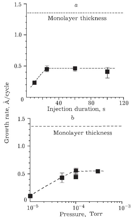
Fig. 10. Temperature modulation Si MLE. Si<sub>2</sub>H<sub>6</sub> injection duration (a) and Si<sub>2</sub>H<sub>6</sub> pressure (b) dependencies. Temperature modulation is 400–550 °C.
