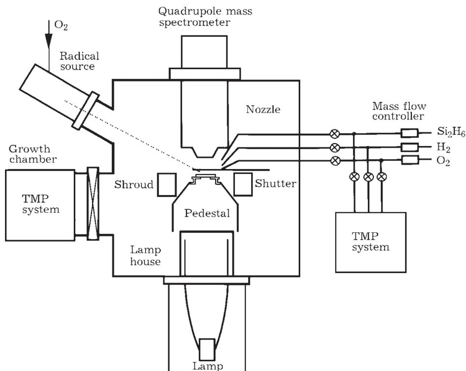
Fig. 8. Si and SiO<sub>2</sub> MLE system.
