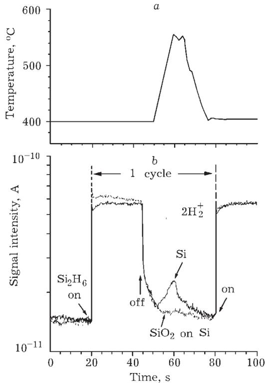
Fig. 9. Time dependence of controlled substrate temperature (a), and *in situ* mass spectroscopic signal of amu  $2H_2^+$  (b).
