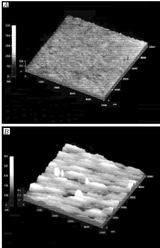
Fig. 2. Growth rate per cycle as a function of growth temperature and the surface roughness observed by AFM. A, B – growth temperature 445 and 514 °C, respectively.
