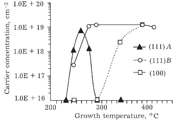
Fig. 3. Te doped crystallographic orientation dependence on the carrier concentration.  $P$ , Torr:  $10^{-3}(\text{AsH}_3)$ ,  $7.2 \cdot 10^{-6}$  (TEG),  $10^{-7}$ (DET).
