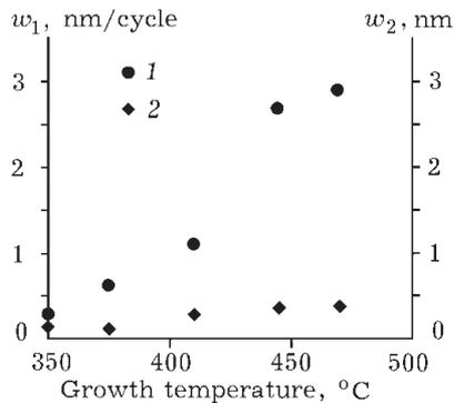
Fig. 7. The lateral growth ( $w_1$ ) in the  $[1\bar{1}0]$  direction and the vertical growth rate ( $w_2$ ) as a function of growth temperature: 1 – lateral growth rate, 2 – growth thickness.
