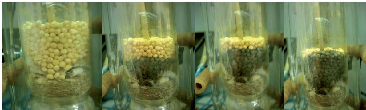
Fig. 1. Dynamics of the solid-phase combustion front propagation in the course of synthesizing the SSTS catalyst 0.4 % Pd/ $\gamma$ -Al<sub>2</sub>O<sub>3</sub> (Pd/CA = 1 : 20). Under the catalyst bed there is ceramics with an electrical coil in order to initiate the process.
