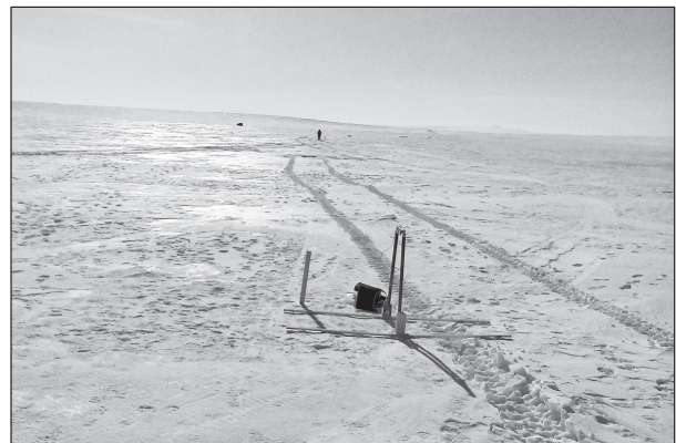
Fig. 2. GROT 12H georadar with antennas of 2 m (75 MHz).
