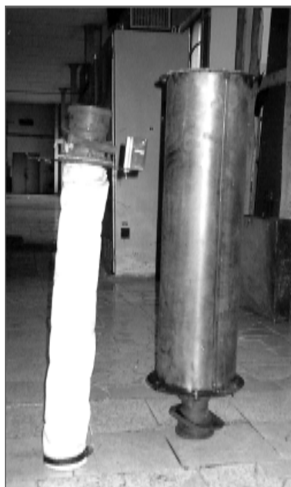
Fig. 4. Visual appearance of the neutralizer with a radial flow of gases (on the right) and of a catalytic glass fibre.
