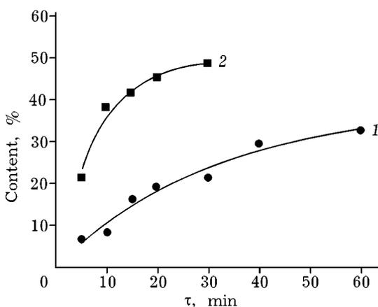
Fig. 2. Changes in the content of water-soluble substances vs. the time of grinding in VTsM (balls) for aspen wood (1) and a mixture of aspen wood with NaOH (2).
