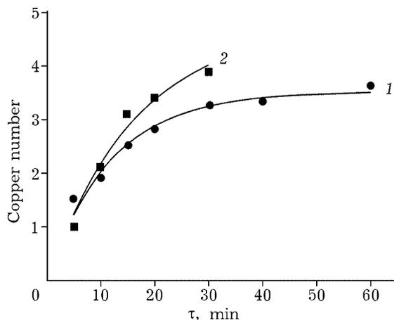
Fig. 1. Changes of copper number for aspen wood (1) and for a mixture of aspen wood with NaOH ( $\text{OH}_{\text{wood}} : \text{NaOH} = 1 : 0.5$ ) (2) vs. the time of grinding in VTsM (balls).
