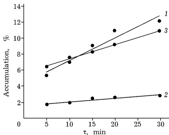
Fig. 4. Accumulation dynamics of monosaccharides present in water-soluble substances of wood after grinding in VTsM in mixture with NaOH: 1 - arabinose, 2 - glucose, 3 - xylose.
