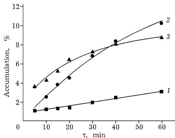
Fig. 3. Accumulation dynamics of monosaccharides present in water-soluble substances of wood after grinding in VTsM: 1 - arabinose, 2 - glucose, 3 - xylose.
