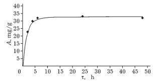
Fig. 3. Sorption kinetics of copper ions on the material of soda-activated bentonite from the Khakasskoye deposit and sawdust modified with a solution of 0.5 M HCl. A – sorption capacity,  $\tau$  – sorption time.
