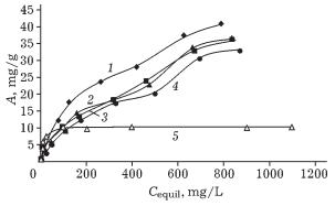
Fig. 2. Dependence of sorption capacity (A) of materials based on bentonite and sawdust on the equilibrium concentration( $C_{equil}$ ) of copper ions in the solution. Modifiers: 1 - 5 % NaOH solution; 2, 3 - 1.0 M (2) and 0.5 (3) M HCl solutions; 4 - 5 % H<sub>3</sub>PO<sub>4</sub> solution; 5 - without modification.
