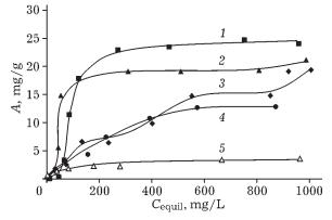
Fig. 1. Dependence of adsorption capacity of modified sawdust (*A*) on the equilibrium concentration ( $C_{equil}$ ) of copper ions in the solution. Modifiers: 1 - 5 % NaOH solution; 2, 3 - 1.0 M (2) and 0.5 M (3) HCl solutions; 4 - 5 % H<sub>3</sub>PO<sub>4</sub> solution; 5 - without modification.
