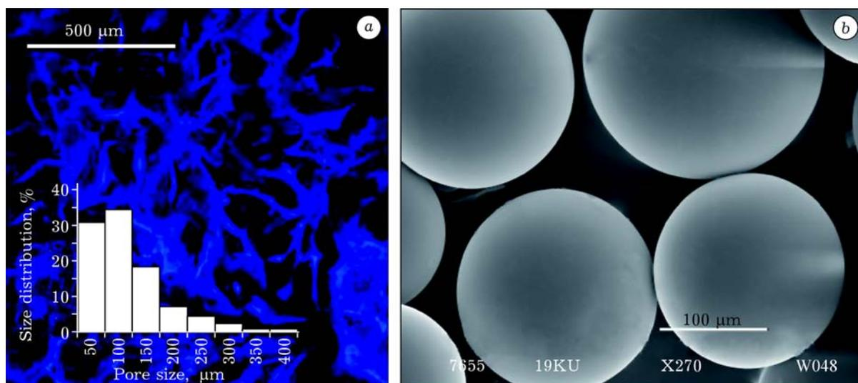
Fig. 3. Different matrix forms for the regenerative medicine based on copolymers of lactide and chitosan: *a* – confocal micrograph of the hydrogel; *b* – micrograph of microparticles obtained using chitosan/lactide samples as an emulsifier.
