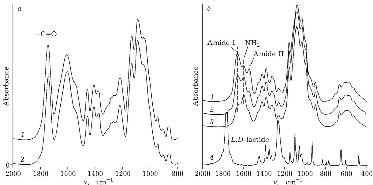
Fig. 2. IR spectra of chitosan/lactide samples obtained at an equimolar ratio between the components at 80 and 90 °C after extracting the unreacted lactide with chloroform (a) and after dialyzing against distilled water (b): 1, 2 - the samples after the treatment at the temperature of 90 and 80 °C, respectively, 3 - chitosan, 4 - *L,D*-lactide.
