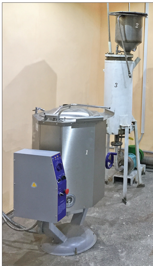
Fig. 2. Enlarged laboratory installation for processing birch bark bast: 1 – reactor ( V = 60 L), 2 – vacuum Nutsche filter ( V = 30 L), 3 – receiver tank ( V = 60 L).
