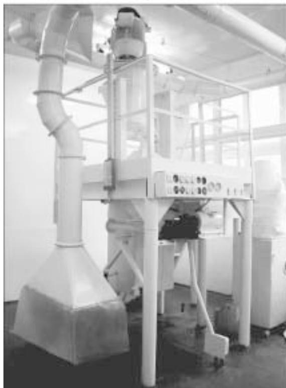
Fig. 15. Schematic diagram (a) and photograph (b) of a mechanical activation set-up for the production of fast-dissolving substances of acetylsalicylic acid.
