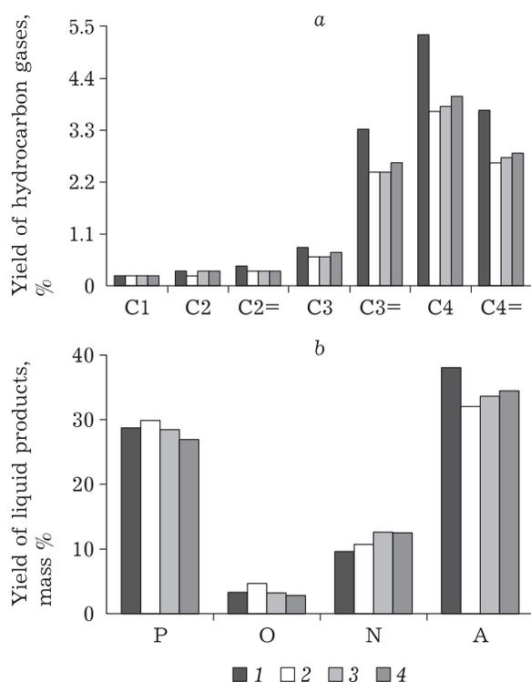
Fig. 1. Composition of hydrocarbon gases (a) and the hydrocarbon fraction of liquid products (b) in cracking of model compounds: VG No. 3 (1); VGO No. 3+ palm oil (2); VGO No. 3 + rapeseed oil (3); VGO No. 3 + sunflower oil (4). P - paraffins; O - olefins; N - naphthenes; A - arenes.
