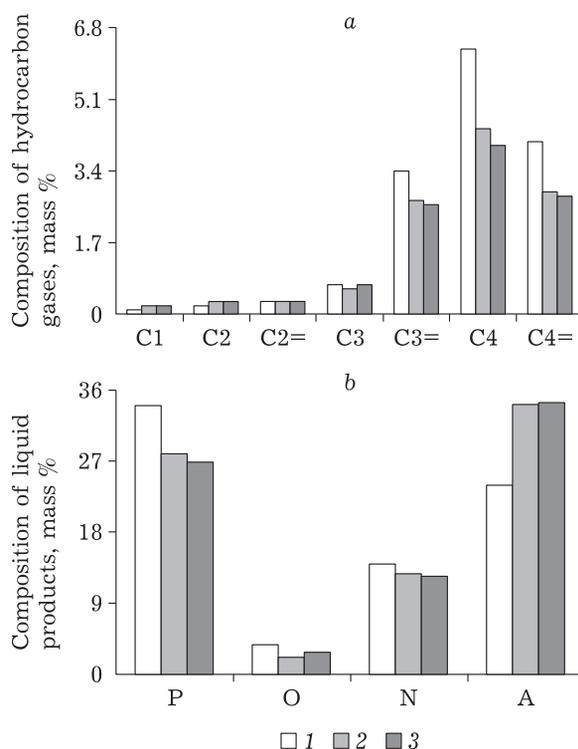
Fig. 2. Composition of hydrocarbon gases (a) and the hydrocarbon fraction of liquid products (b) in cracking of model mixtures with sunflower oil: VGO No. 1 (1); VGO No. 2 (2); VGO No. 3 (3). P - paraffins; O - olefins; N - naphthenes; A - arenes.
