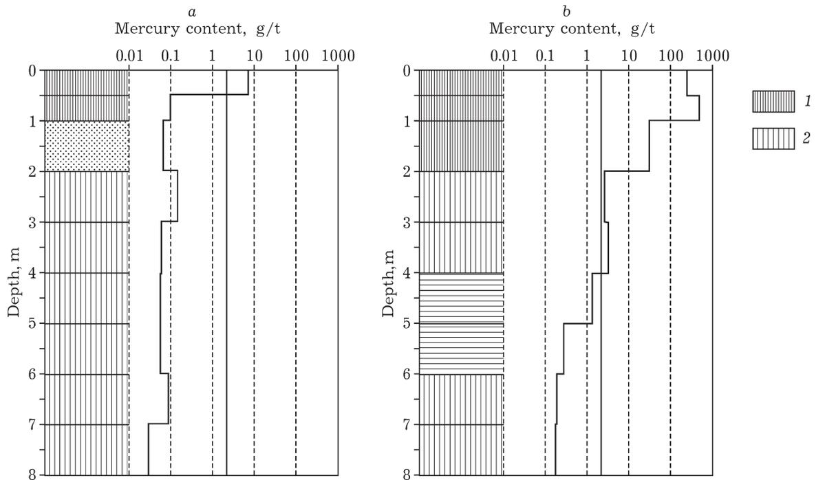
Fig. 3. Mercury content in soil sections according to typical boreholes Nos. 13 (*a*) and 12 (*b*) in the central part of the industrial area at the JSC NCCP: 1 – soil, 2 – man-caused soil layer. Thick line shows the MPC value in soil (2.1 g/t).
