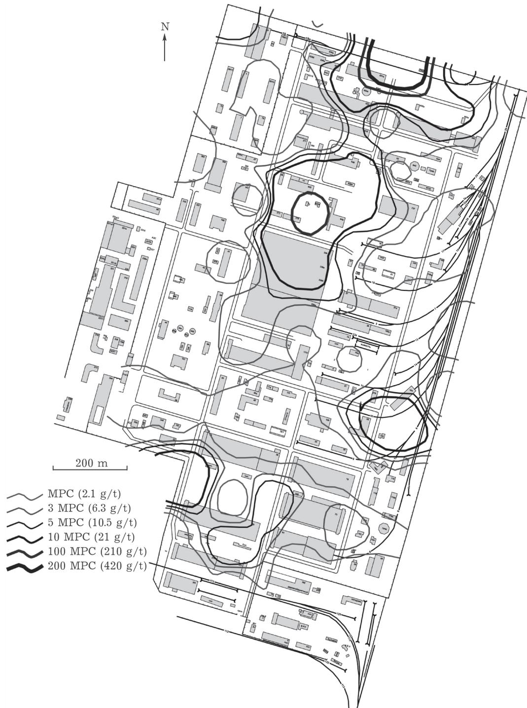
Fig. 4. Mercury anomalies in the surface man caused soil layer the industrial area at the JSC NCCP. Compiled by A. G. Vladimirov, I. M. Belozerov and S. V. Vystavnov.
