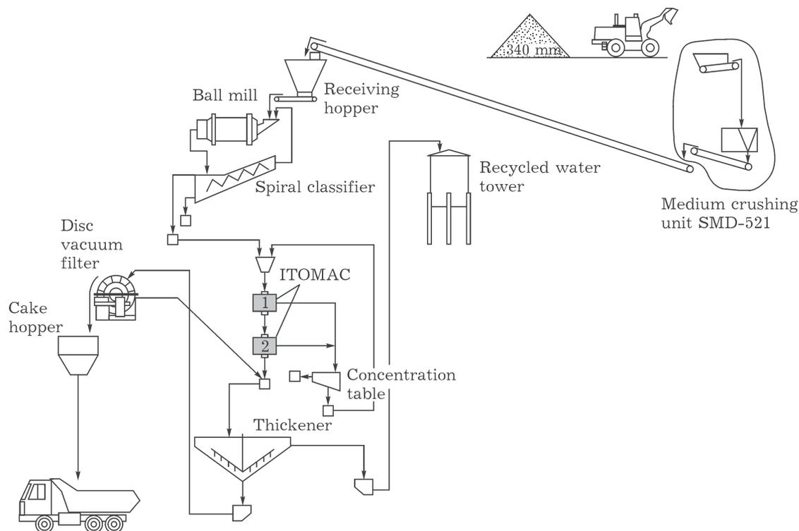
Fig. 5. Flow sheet for processing solid mercury-containing wastes and building materials at the chemical and metallurgical production sector of the NCCP. Compiled by A. V. Babushkin, I. M. Belozyorov, A. G. Vladimirov, V. A. Minin.
