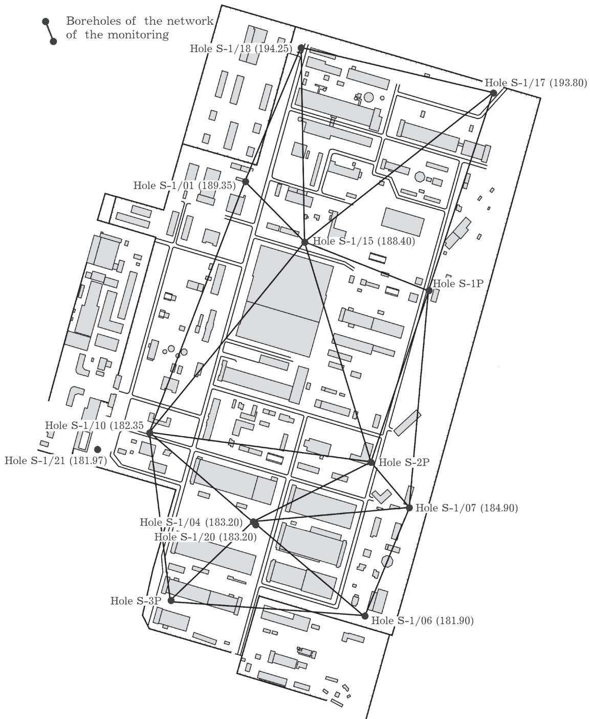
Fig. 1. Industrial area of the JSC NCCP and the network of the monitoring ecogeochemical and hydrogeological boreholes.
