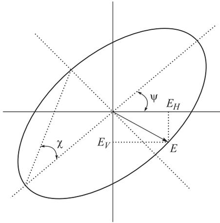
Fig. 1. Polarization ellipse.
