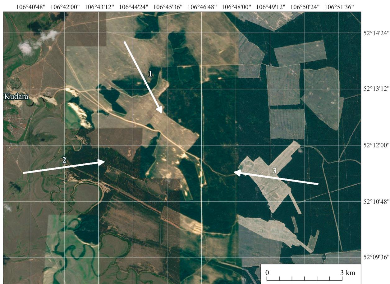
**Fig. 3.** Test area on the Google Maps and geometry of radar imaging for SIR-C (arrow 1) and ALOS PALSAR at ascending (arrow 2) and descending (arrow 3) orbits.
