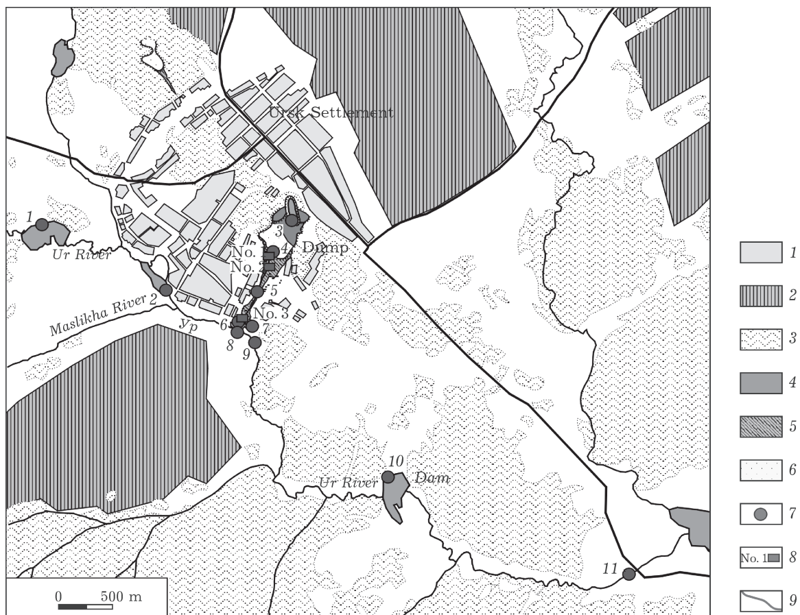
Fig. 1. Scheme of the Urskoye tailing dump, adjacent territory and sampling sites for surface water and solid matter: 1 – residential areas of Ursk settlement; 2 – tillage; 3 – forest; 4 – rock debris; 5 – zone of carried waste material; 6 – tailing dump; 7 – surface water sampling sites; 8 – trenches; 9 – automobile roads; 10 – dam near the dredge; 11 – Ur River.
