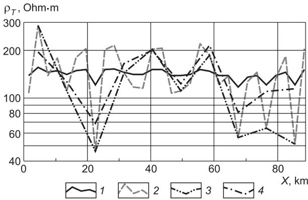
**Fig. 6.** Charts of  $\rho_T$  on a period of 36 s. 1, one-dimensional curves at reference points; 2–4, transverse curves for the following models: 2, A with a step of 1 km; 3, A with a step of 3 km; 4, B with a step of 3 km.
