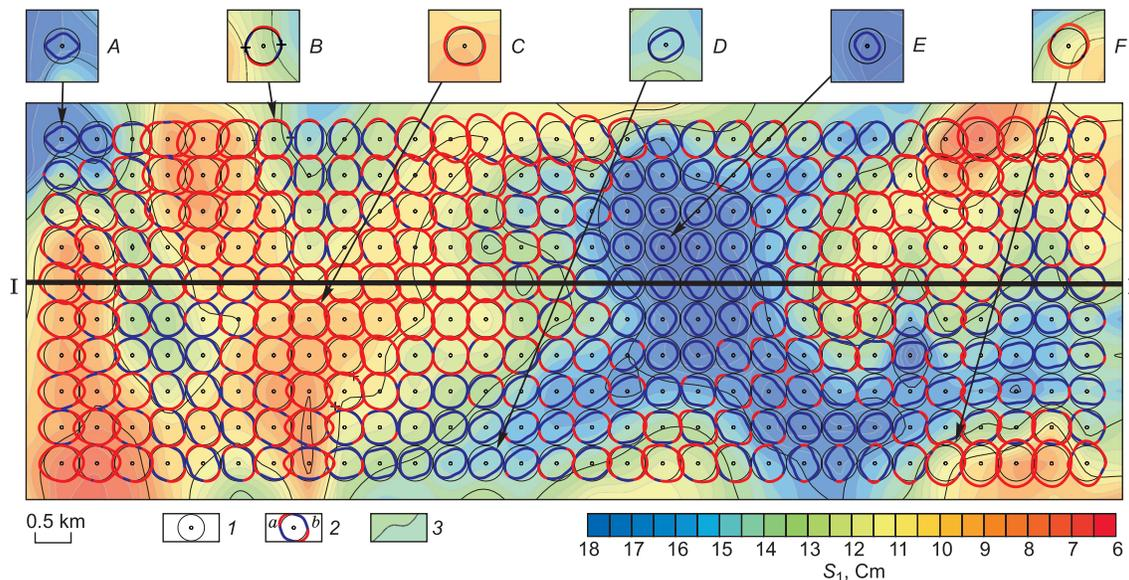
**Fig. 3.** Calculation results for the azimuthal distribution  $K_{gs}$ . 1, MTS reference points and the unit circle; 2, azimuthal diagrams  $K_{gs}$ : a,  $K_{gs} > 1$ , b,  $K_{gs} < 1$ ; 3, conductivity isolines. The inset above: A, complex-shaped azimuthal diagrams; B, the effective curve is not deflected in level; C, all curves are above the normal level; D, the maximum curve is not deflected; E, all curves are below the normal level; F, the minimum curve is not deflected.
