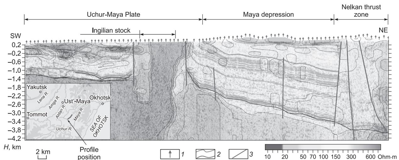
Fig. 8. Seismological section. 1, MTS points; 2, reflecting boundaries; 3, tectonic faults.
