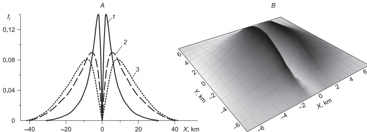
**Fig. 1.** Filter shape for the formation of  $S_e$ : two- (A) and three-dimensional (B) versions. 1–3, the shape of the two-dimensional filter with the following position of the inhomogeneity: 1, above the screen, 2, below the screen with moderate transverse resistance ( $< 1 \cdot 10^7$  Ohm·m<sup>2</sup>), 3, below the screen with high transverse resistance ( $> 10 \cdot 10^7$  Ohm·m<sup>2</sup>).
