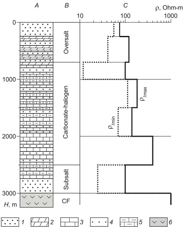
**Fig. 2.** Geological (A and B) and geoelectric (C) models of the area under study. 1, sandstones; 2, marls; 3, limestones and dolomites; 4, salts; 5, mudstones and siltstones; 6, crystalline rocks of the basement;  $\Phi$ , crystalline basement,  $\rho_{l\min}$  and  $\rho_{l\max}$  denote the approximate minimum and maximum longitudinal resistances of the horizons.
