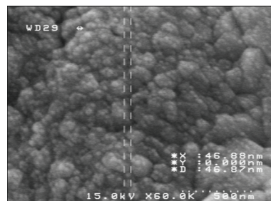
Fig. 3. SEM image of ZnO nanostructure prepared by the thermal decomposition of compound 1 with oleic acid as a surfactant at 180 °C
