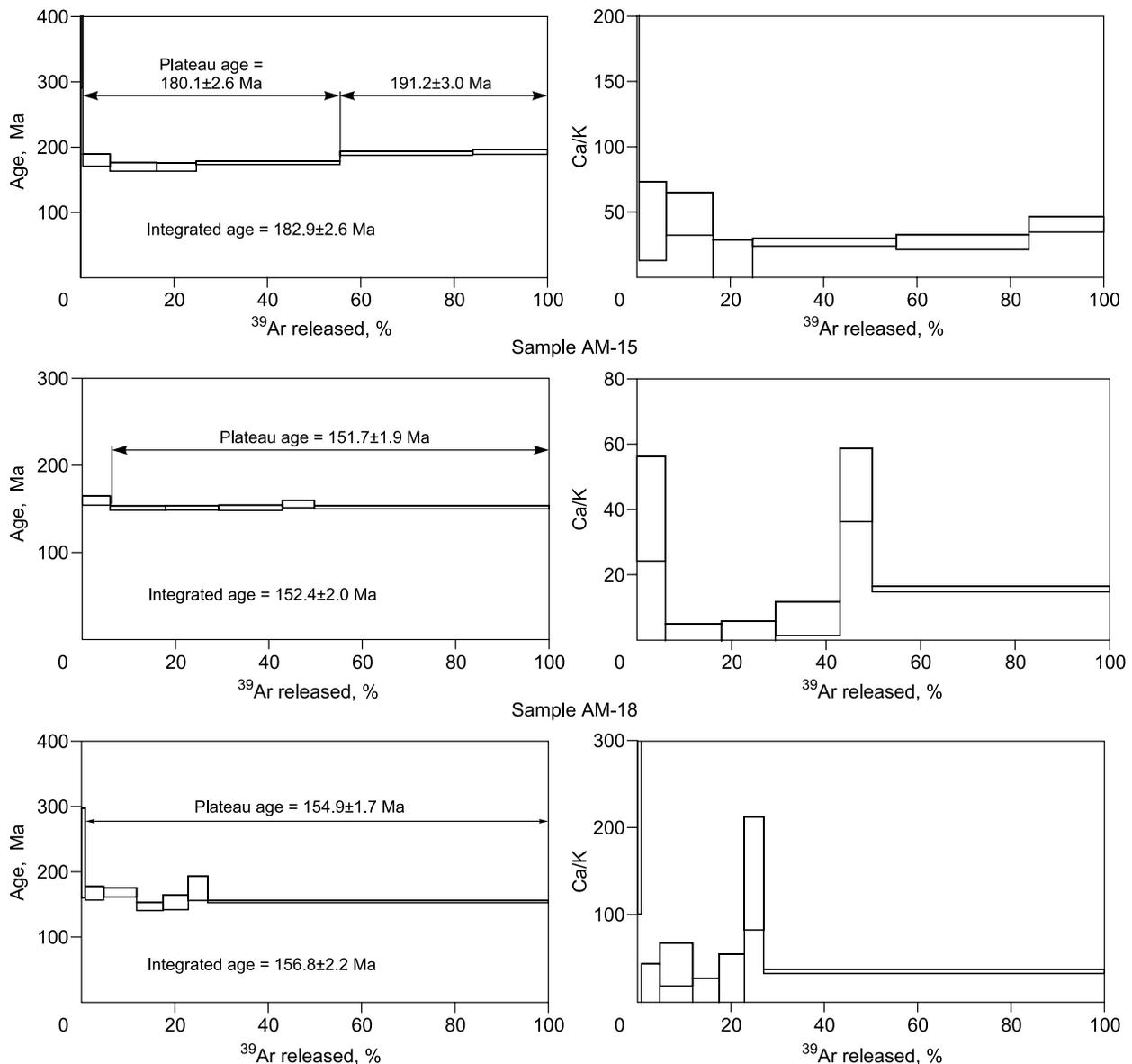
**Fig. 3.** Results of Ar/Ar dating of Mesozoic granitoids of the Kara gold ore cluster. For explanation, see the text.
