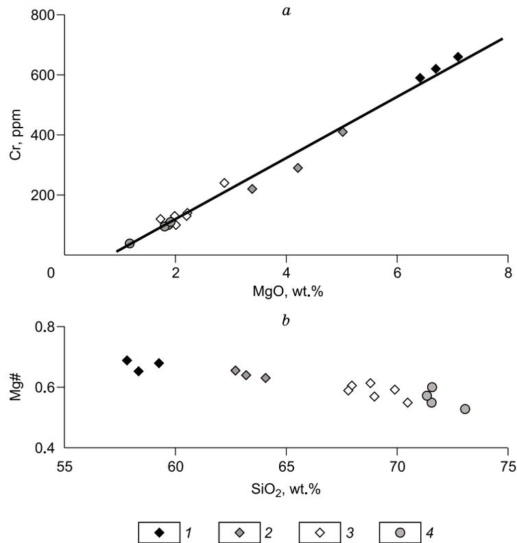
**Fig. 6.** Cr–MgO (a) and Mg#–SiO<sub>2</sub> (b) diagrams for granitoids of the Amudzhikan–Sretensk complex. Mg# =  $Mg^{2+}/(Mg^{2+} + Fe^{2+} + Fe^{3+})$ . Composition of rocks: 1, hybrid porphyry; 2–4, granitoids of: 2, first, 3, second, 4, third phases.
