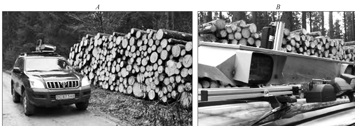
Fig. 3. Mobile camera log measurement system by the Dralle company: A – general view; B – the measurement unit (Dralle, 2015).
