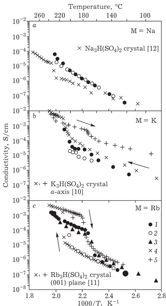
Fig. 3. Temperature dependence of conductivities of  $M_3H(SO_4)_2$  prepared by milling and *via* solution process for comparison: 1–3 – denote the 1st cooling, 2nd heating and 2nd cooling of the samples prepared by milling, respectively; 4, 5 – the 1st heating and cooling of  $M_3H(SO_4)_2$  prepared *via* solution process [10–12].
