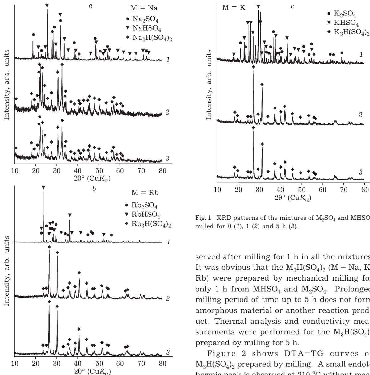
Fig. 1. XRD patterns of the mixtures of  $M_2SO_4$  and  $MHSO_4$  milled for 0 (1), 1 (2) and 5 h (3).
