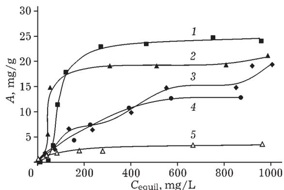
Fig. 1. Dependence of adsorption capacity of modified sawdust ( $A$ ) on the equilibrium concentration ( $C_{\text{equil}}$ ) of copper ions in the solution. Modifiers: 1 – 5% NaOH solution; 2, 3 – 1.0 M (2) and 0.5 M (3) HCl solutions; 4 – 5%  $H_3PO_4$  solution; 5 – without modification.
