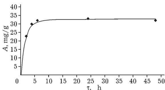
Fig. 3. Sorption kinetics of copper ions on the material of soda-activated bentonite from the Khakasskoye deposit and sawdust modified with a solution of 0.5 M HCl.  $A$  - sorption capacity,  $\tau$  - sorption time.
