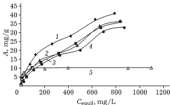
Fig. 2. Dependence of sorption capacity ( $A$ ) of materials based on bentonite and sawdust on the equilibrium concentration ( $C_{\text{equil}}$ ) of copper ions in the solution. Modifiers: 1 - 5% NaOH solution; 2, 3 - 1.0 M (2) and 0.5 (3) M HCl solutions; 4 - 5%  $\text{H}_3\text{PO}_4$  solution; 5 - without modification.
