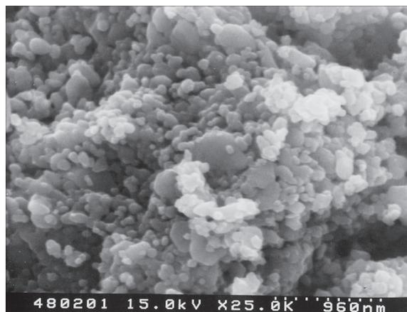
Fig. 7. SEM image of the calcined product after grinding the mixture of ZnO and 5 % urea for 1 h.
