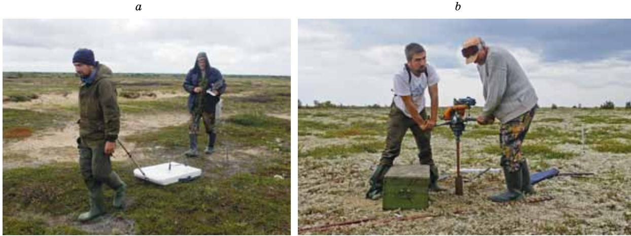
Fig. 2. GPR profiling (a) and coring (b) in the study area.
