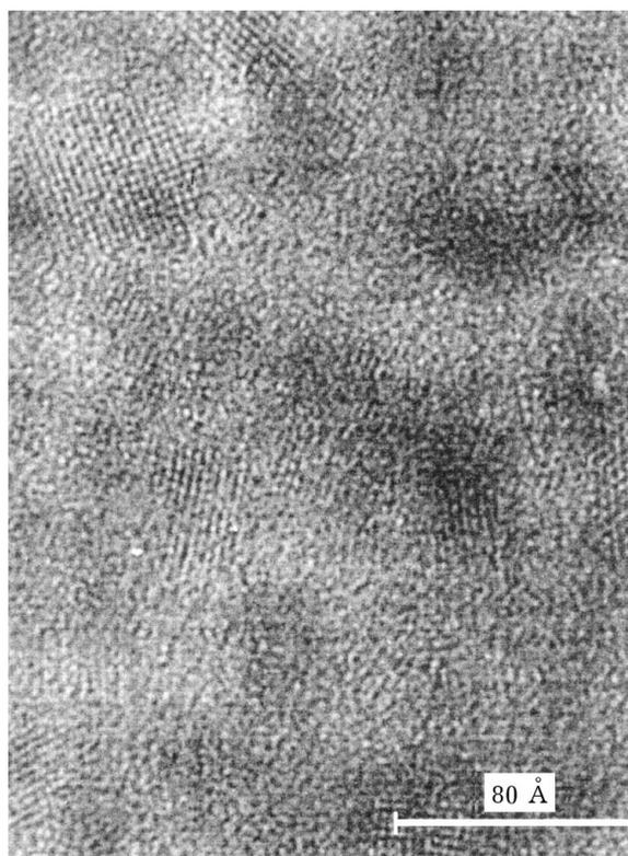
Fig. 2. HREM image of PbS nanoclusters in the matrix of behenic acid.
